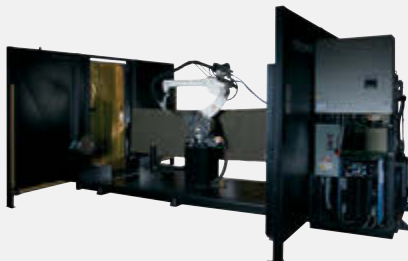
Robot between dual head and tailstock/single- or dual-robot configuration
