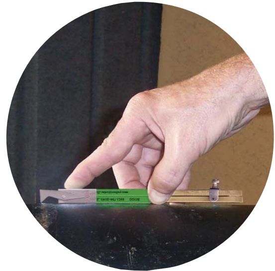
The Pit Depth Gauge can be used to check weld undercut and misalignment of plate to plate or pipe to pipe.
