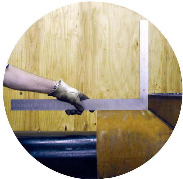
The D241 Large Framing Square and D256 Small Framing Square can be used to check squareness of pipes, flanges, and fittings.
