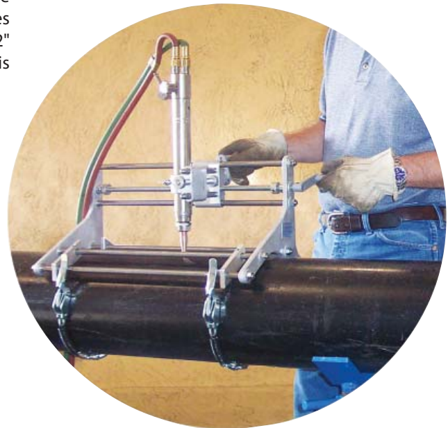
An excellent tool for making coupons for bend test, tensile test, and hardness tests.
