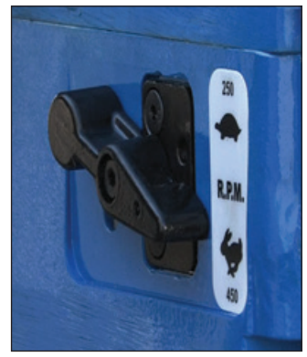
Two speed gear box for increased tool life
